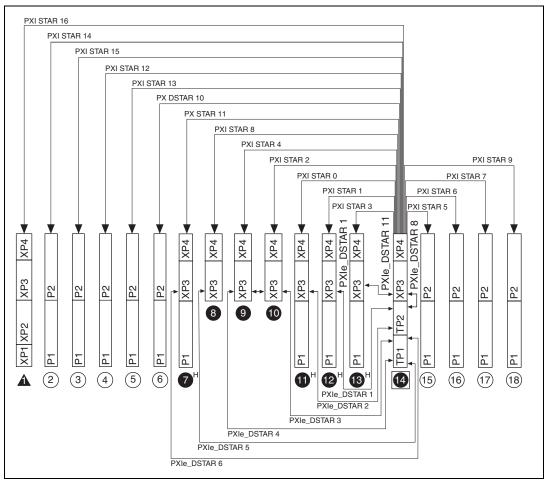
Figure 1-3. PXIe\_DSTAR and PXI Star Connectivity Diagram
